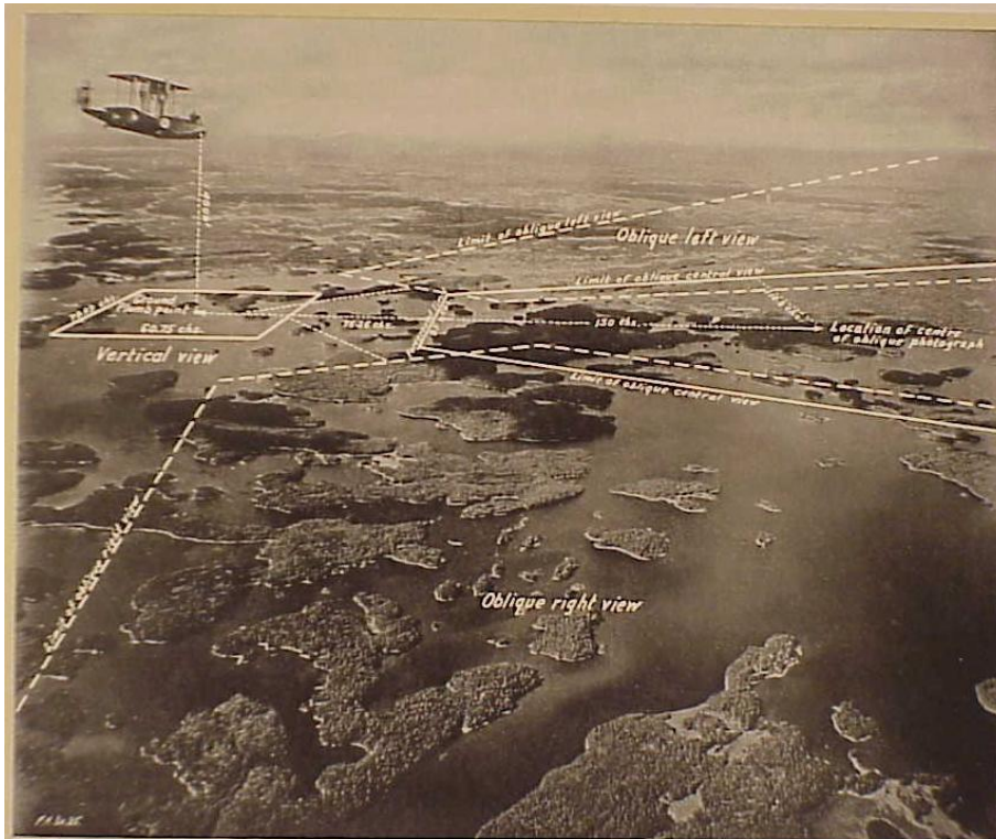
Oblique Aerial Mapping View, illustrating method of oblique photographing for mapping purposes. The relative
