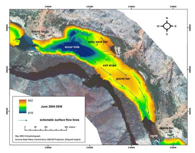
Figure 2. Map of a debris fan-eddy complex in lower Marble Canyon (river mile 43.5 to 44.0) showing the characteristic features of this fundamental channel unit.
