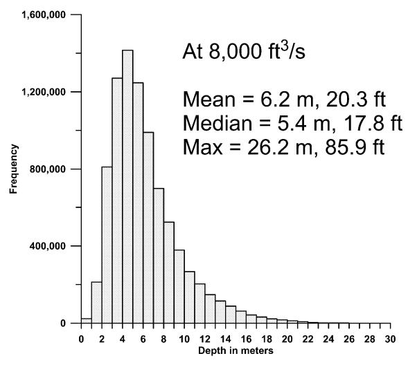
Figure 1. Histogram of river depths at a flow of 8,000 ft<sup>3</sup>/s.
