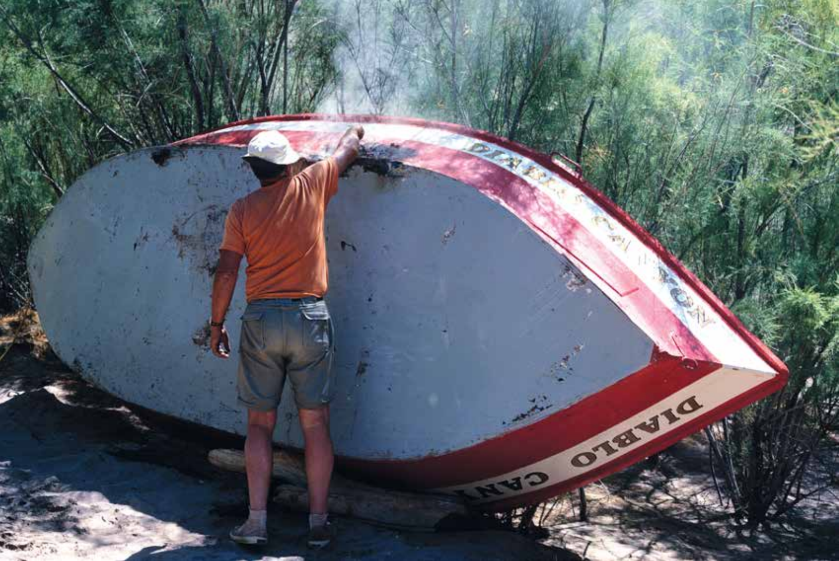
Boat repair at Bass—Martin Litton building a fire in a frying pan to dry out the wet wood. Photo: John Blaustein
