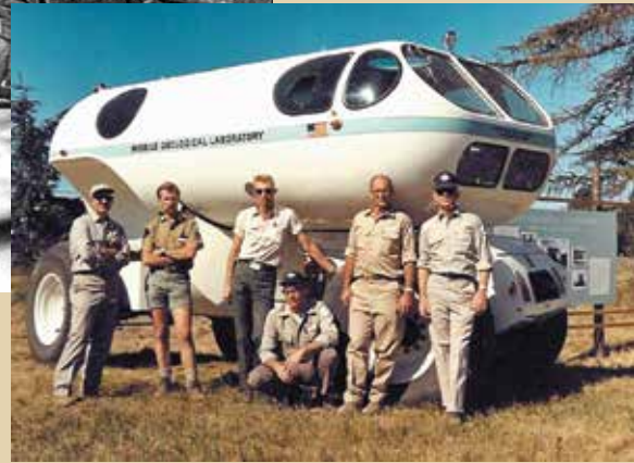
Mobile Laboratory (MOLAB) or Mobile Geologic Laboratory (MGL) designed for NASA by General Motors in 1965 for NASA as a prototype, extended lunar mission vehicle; (a) (l to r) Hal Stephens, Ivo Lucchitta, Bill Tinnin, Bob Sutton and two others (unidentified) standing in front of MOLAB; USGS photo USGS Open-File Report 2005-1190, Figure 023a.
