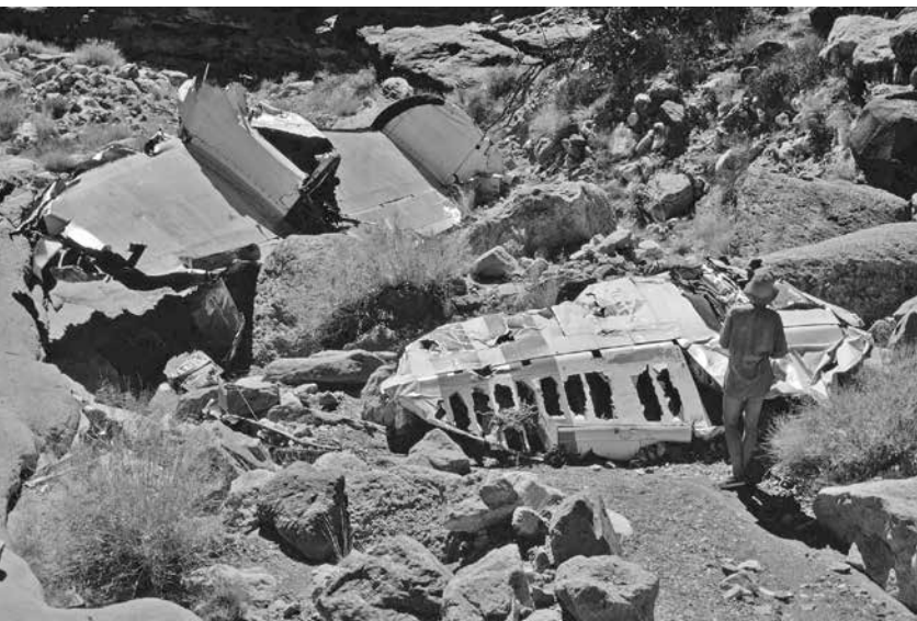
Tail of the TWA Constellation airliner from the 1956 air crash. Note the probable propeller damage from the collision with the United Douglas DC-7. Temple Butte area, Grand Canyon. NAU.PH.2004.B.2.32.21 Margaret Eiseman Collection
