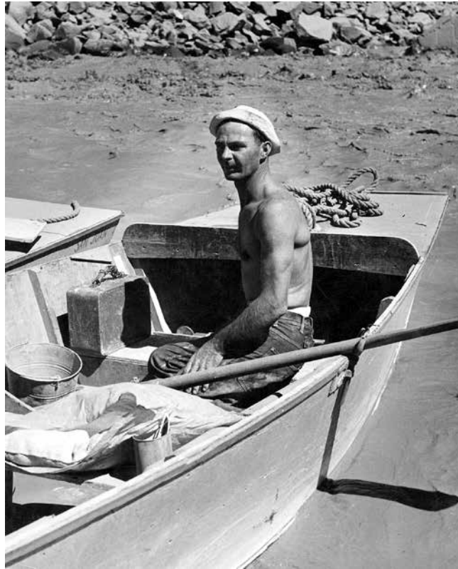
By the mid-1940s, the Nevills San Juan boats had abandoned the horse trough design and were following the lines of the cataract boats—five feet wide at the gunwales with about ten inches of rake at bow and stern. These refinements allowed the boats to carry more passengers and made them much more maneuverable.
