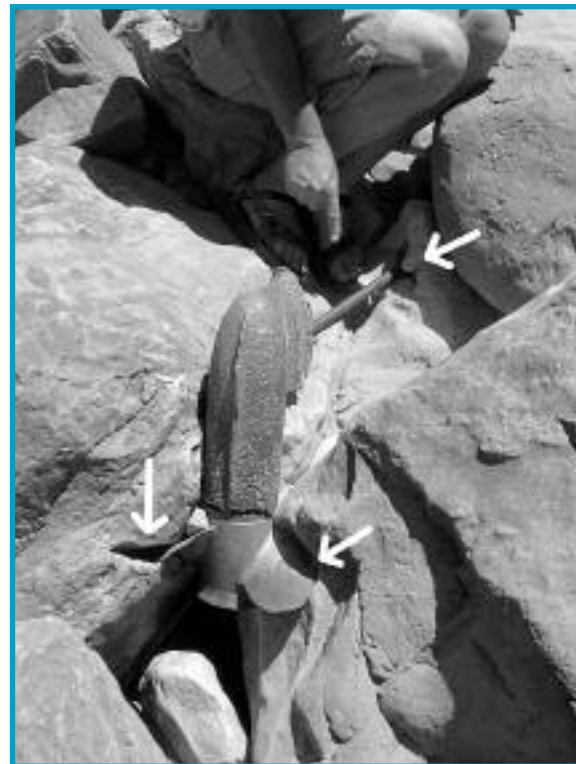
Figure 2—2002—Lower unit of an outboard motor sutured into a rock at Rapid 7, Cataract Canyon. The propeller blades have sliced into two boulders, and the drive shaft, free to rotate, has cut a horizontal slot into another boulder.
